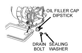
Figure 22. Engine Oil (Draining)
